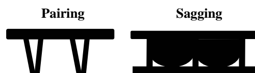
Fig. 4. Pairing and sagging of a PDMS stamp.
